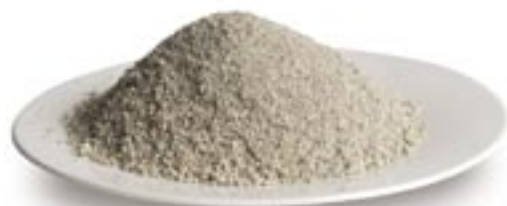
Figure 3 Granulated Blast Furnace Slag
