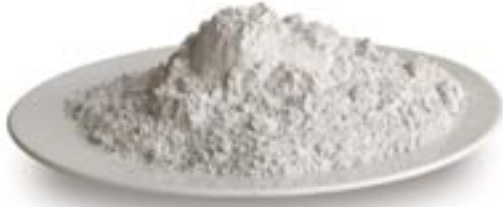
Figure 4 Ground Granulated Blast Furnace Slag
