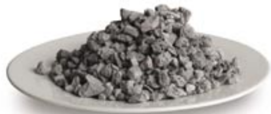
Figure 2 Air Cooled Blast Furnace Slag Aggregate
