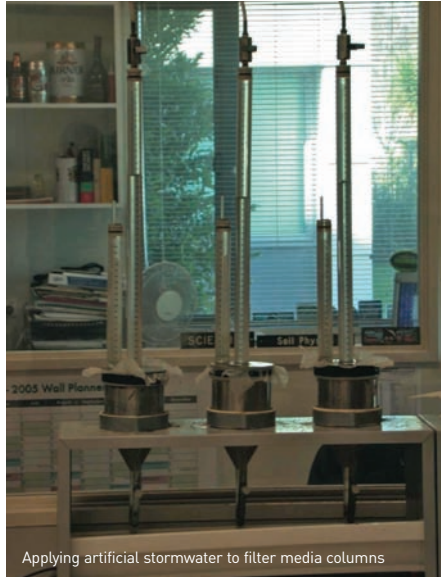
Measuring hydraulic conductivity of filter media using disk permeameters
