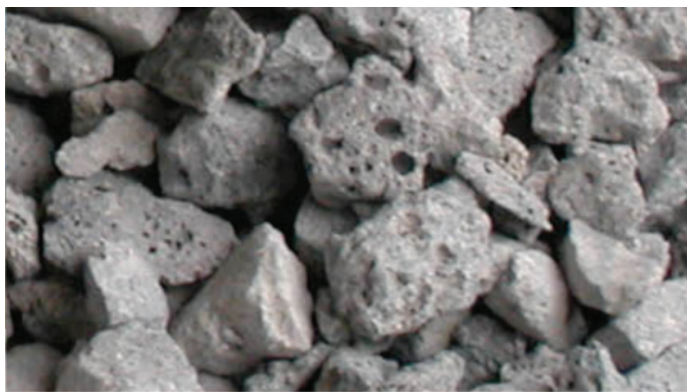
Figure 1 - Blast Furnace Slag Aggregate (10mm-20mm size)
